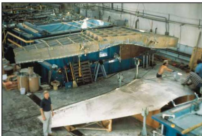
**Figure 6** Electroformed nickel mould for wing skins for Harrier Jump-jet.
