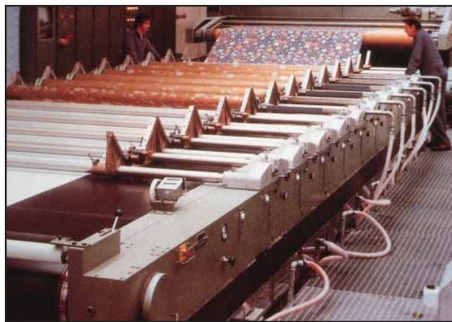
**Figure 4** Textile printing machine using electroformed nickel screens.
