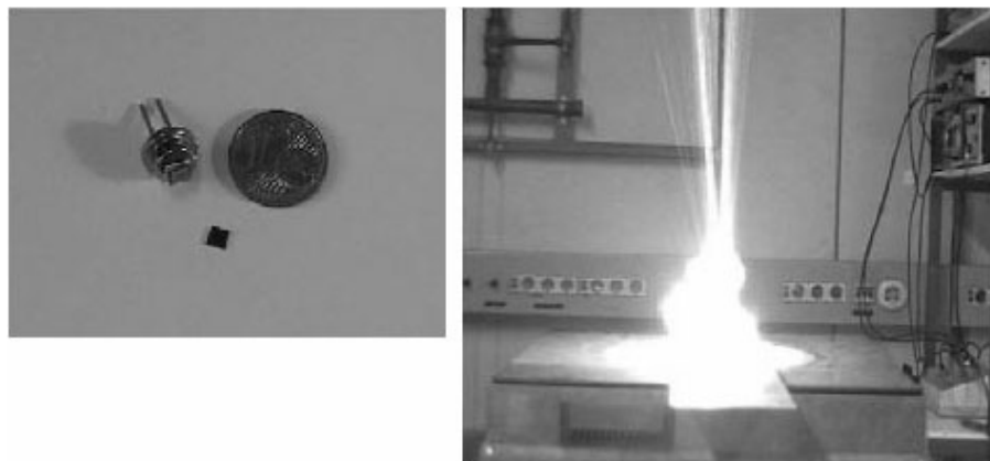
Fig. 4 Left side: Picture of a single PSI-based explosive element (bottom), a prototype of the airbag igniter (upper left) in comparison with a Eurocent coin. Right side: Image of the ignited single explosive element.
