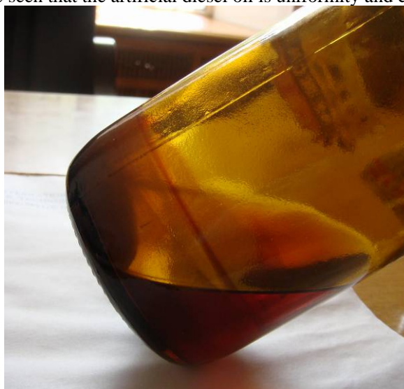
Fig. 3 Artificial diesel oil after 13 years deposition
